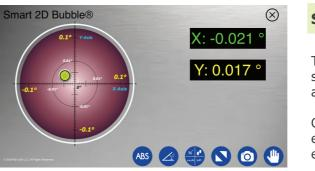
Smart 2D Bubble<sup>\*</sup>, view on smartphone or tablet screen using mobile sync app
